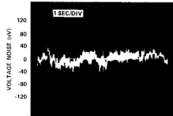
0.1Hz TO 10Hz PEAK-TO-PEAK NOISE
